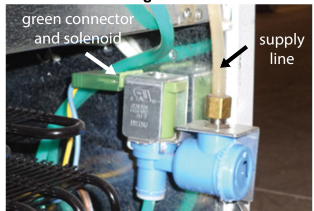
Single Water Valve (supply line, green connector, and solenoid shown)
